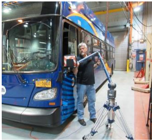
Figure 4. VTTI scanned a transit bus at the NYCT DOB to produce a reverse engineering model for FTA Report No. 0219.
