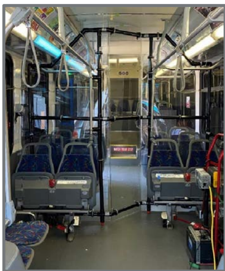
Figure 9. A prototype mid-bus barrier developed and installed in a transit bus for air flow testing on the Virginia Smart Roads test bed for FTA Report No. 0224.
