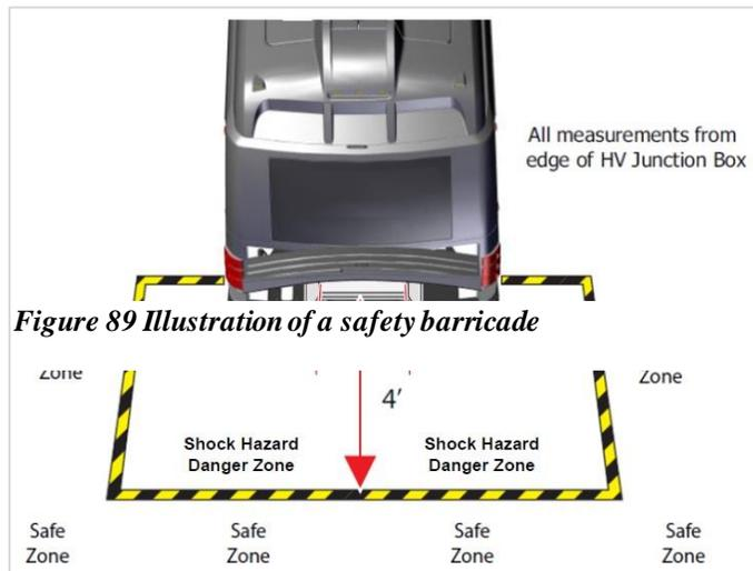
*Figure 89 Illustration of a safety barricade*
