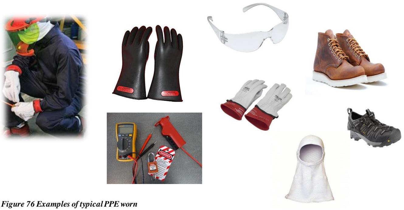
Figure 76 Examples of typical PPE worn during BEB maintenance
