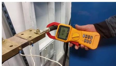
*Figure 85 Clamp-on current probe*
