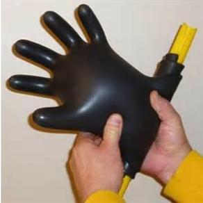
Figure 79 Manual glove inflation inspection
