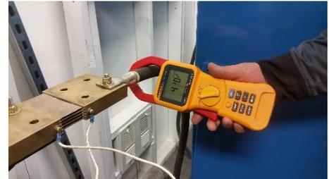
*Figure 85 Clamp-on current probe*
