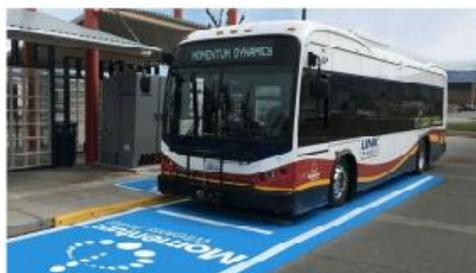
*Figure 94 Example of a wireless charging bus*
