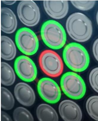
Passive Propagation Resistance [PPR] is a safety feature within the batteries modules/ESS. The feature of PPR allows individual cell units within the battery to be encased in a specialized foam material, which acts as a strong isolator material in-between the cells.
