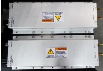
Figure 15 DC to DC converter
