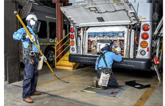
*Figure 1 Technicians performing maintenance on a BEB*
