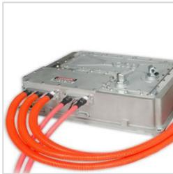
Inverters are used to change the DC voltage stored in the high voltage batteries to 3-phase alternating current [AC]. The AC voltage is supplied to an electric motor to generate movement. BEBs will have multiple inverters to perform different tasks, such as powering an air compressor, HVAC, or turning the traction motors.
