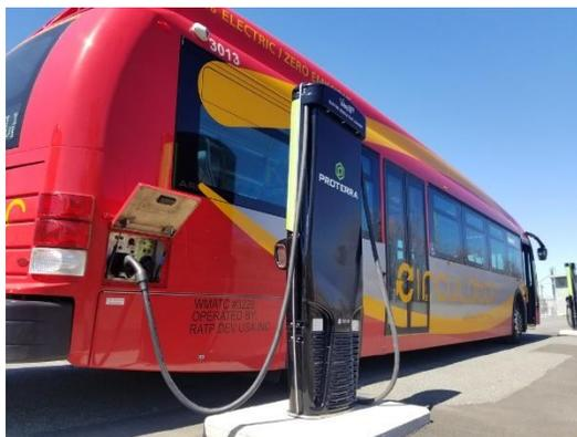
This is the currently the most common method of BEB charging, and the type of infrastructure you will likely find in a transit agency. With overhead, the infrastructure will include a charger and a charge post or dispenser. The two types are:
