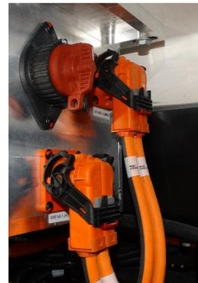
Figure 18 HV Cables
