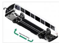
It is absolutely vital to a BEB that regenerative braking be working efficiently. As mentioned, it is a process that begins anytime the driver starts to reduce acceleration, and turns the motor into a generator and try and recuperate that energy. In that regard it kind of works like a hybrid, as we decelerate, trying and recover some of that power.
